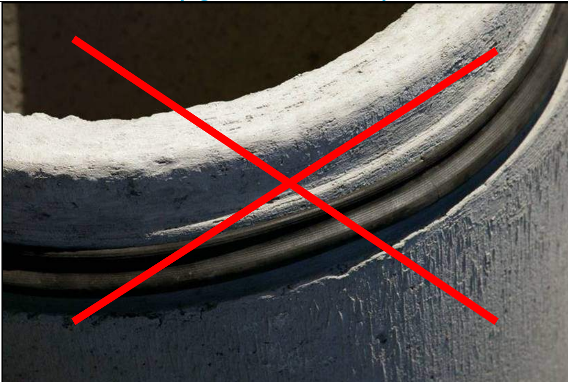
INCORRECT POSITIONING OF GASKET
