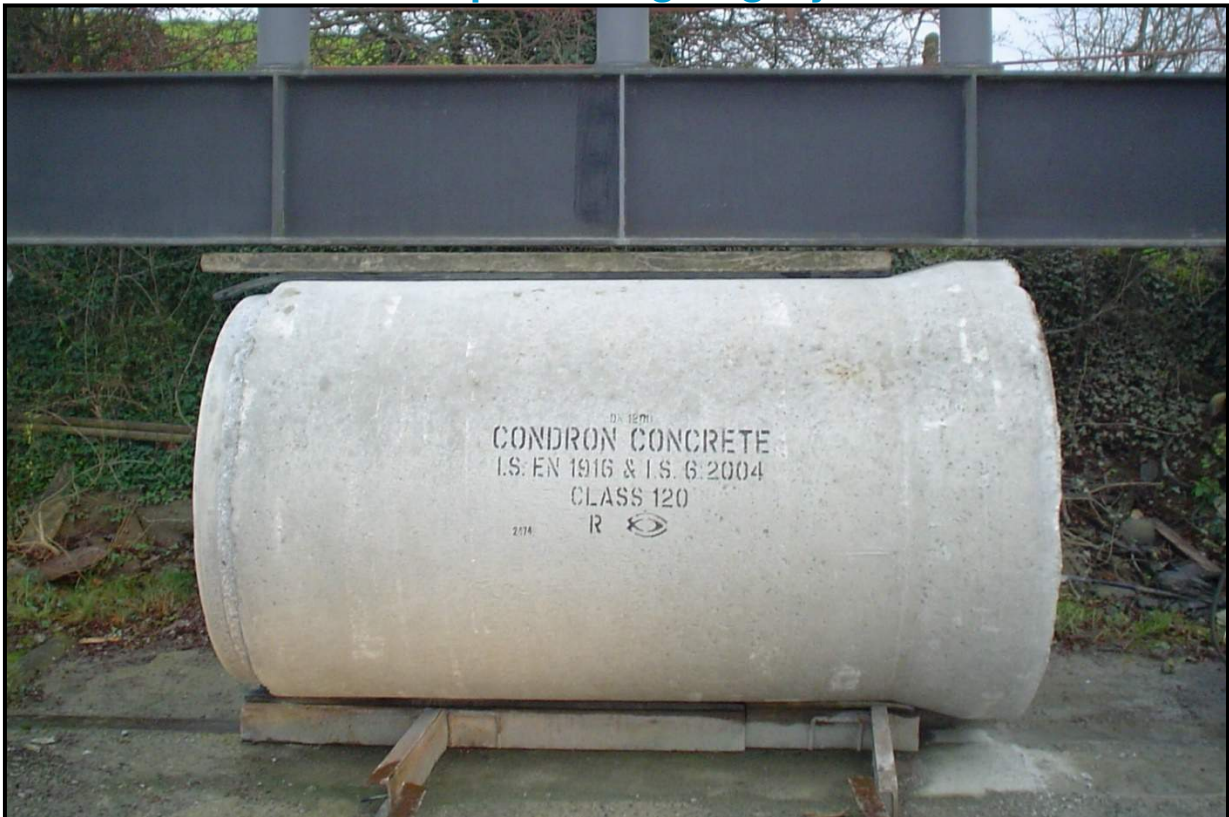
1200mm \varnothing I.S. 6 Pipe undergoing Crush Test
