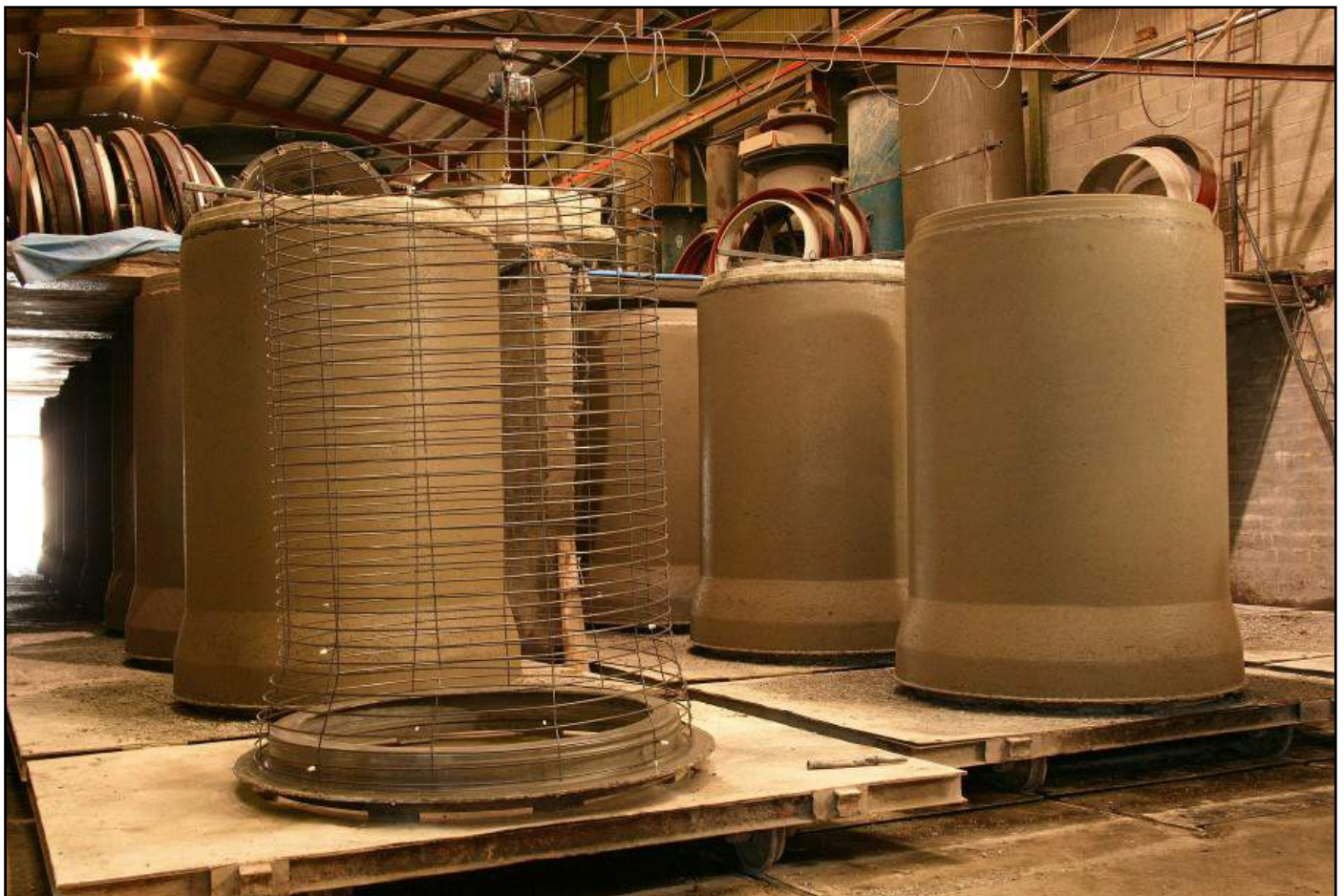
Reinforcement Cage for 1500ø I.S. 6 Pipe
