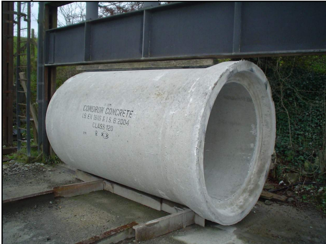
1200mm \varnothing I.S. 6 Pipe undergoing Crush Test
